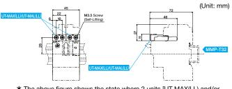
\* The above figure shows the state where 2 units [UT-MAX(LL) and/or UT-MAL(LL)] are installed.
