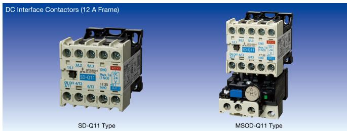
Direct Drive of Contactors Using Semiconductor Output (Transistor Output) Can drive a direct DC interface contactor using DC24 V transistor output without use of an intermediate relay.
