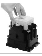
(2) Insert the lever of the auxiliary contact unit (UN-AX80) into the window of the contactor side, and bring it into close contact with the contactor.
