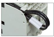
\* The magnetic relays have the wire holders for the outermost poles.
