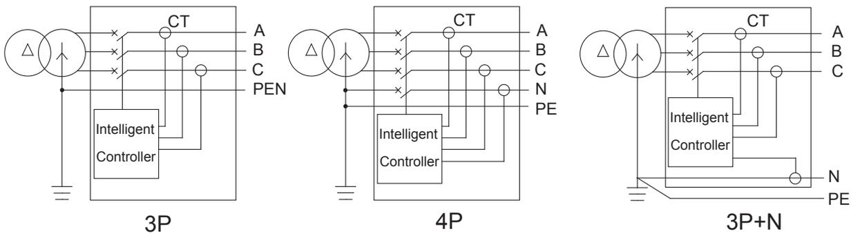
Grounding current: Measure current between phase line and neutral in a TN-S system, measure in the Neutral - earth link of the LV transformer (shown below), when there is a grounding fault, PE line will generate current, causing fault determined.
