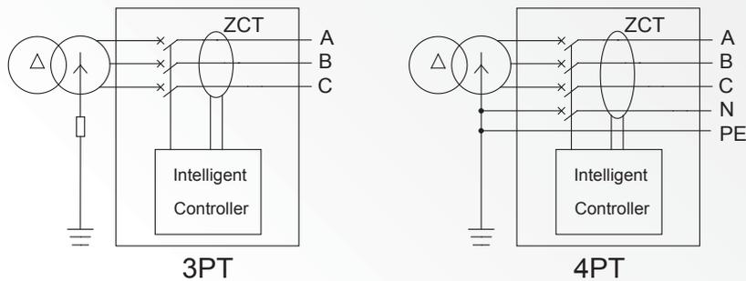
**■ Ground fault alarm/ Earth leakage alarm/ Overload pre-alarm**
