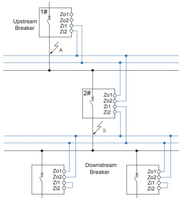
Zone-selective interlocking (ZSI) has multiple classified protection system which is designed to minimize the faulty impact on whole electrical distribution system by reducing the time it takes to clear the fault and maintaining system coordination. This function is suit with short circuit and ground fault protection ( $I^2t$  is set to off)
