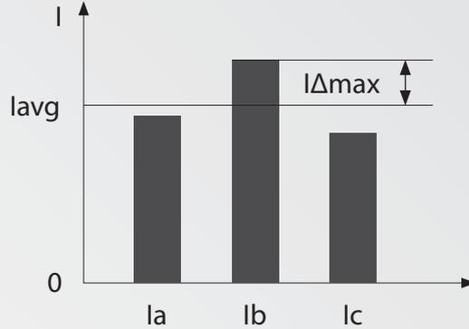
In the equation,  $I_{avg}$  :  $I_a, I_b, I_c$  3 phase average current (RMS).  $I \Delta_{max}$  : maximum difference of each phase and  $I_{avg}$ .
