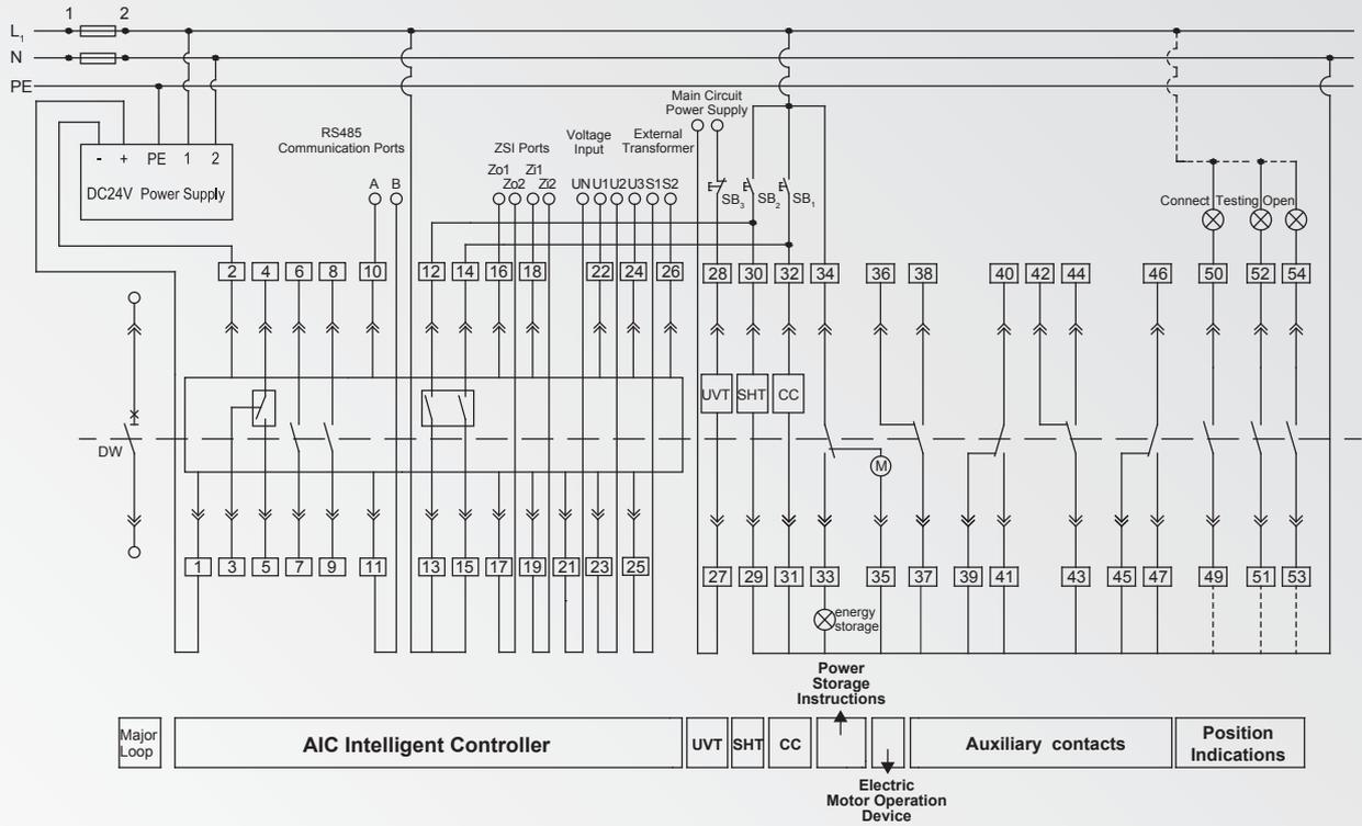
Note: Set the first set of programmable contact (12 # , 13 # ) "remote open" and pair with a SHT ; set the second programmable contact (14 # , 15 # ) to "remote close" and pair with a CC ; then use the controller to send out signal for remote control.
