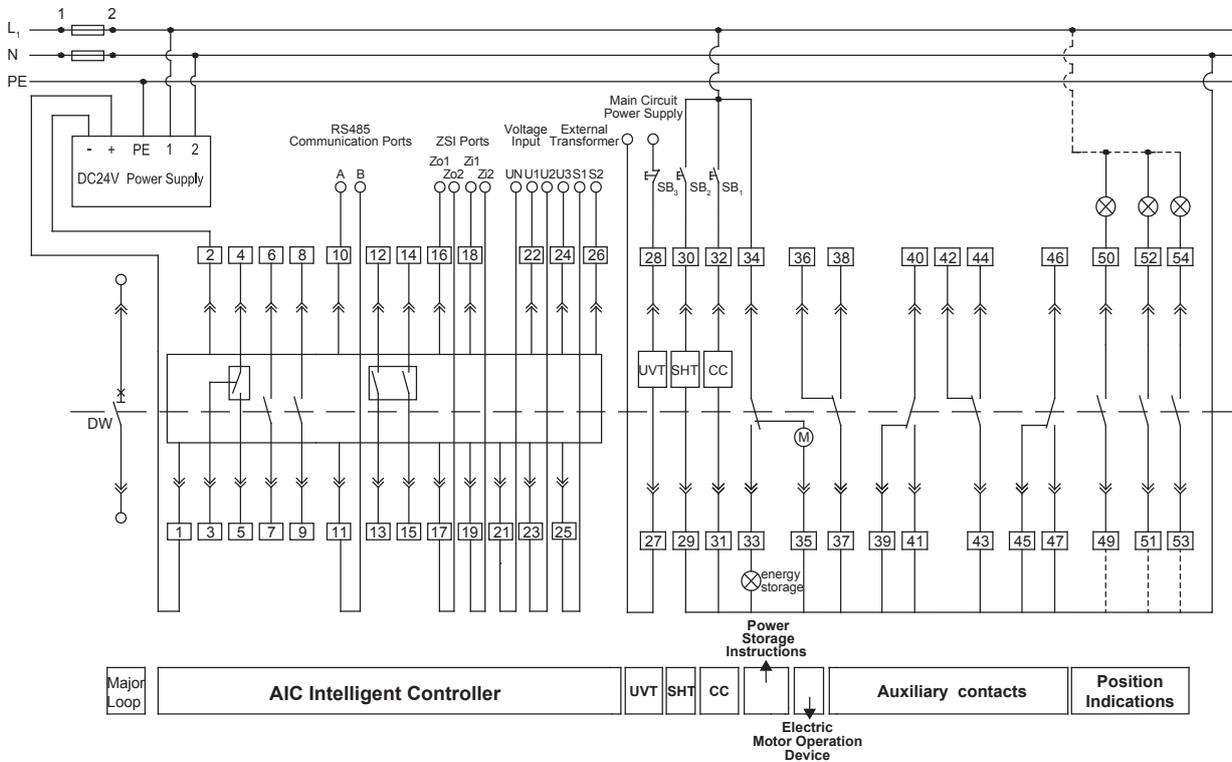
Note: (1) If CC, SHT and M are using different control voltage, they should connect to different power source.
