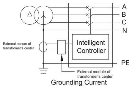
Note: TN-S is 3 phase 5 wires, including A、B、C、N、PE.
